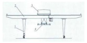
The weight of the container is measured using a hanging apparatus that measures the amount of weight exerted on each handle holding the container.
